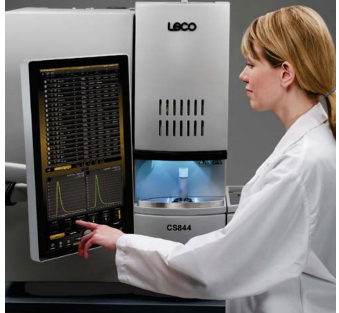
LECO carbon analyzers are a rapid alternative to the C311 Loss on Ignition test method. (Photo: LECO Corporation)
