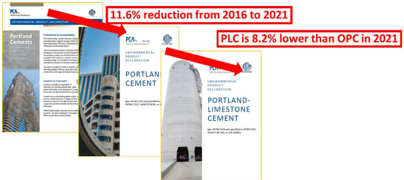
Figure 2. PCA’s industry-average EPDs show progress in reducing the GWP of portland cement from 2016 to 2021, as well as the average reduction in GWP for portland-limestone cement compared to portland cement.
