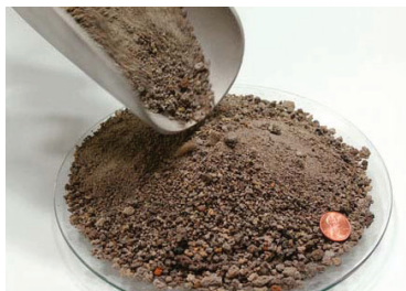
Bottom ash is a granular material suitable for replacing gravel and sand.
