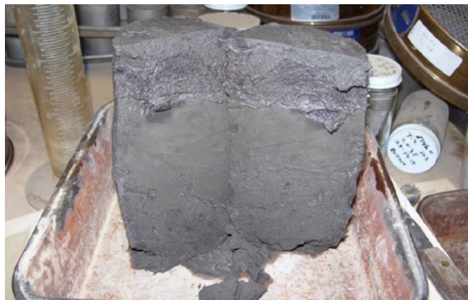
Fine-particle CCRs in layers, showing excess porewater. This type of free liquids/porewater can be removed by dewatering. The containment of the porewater measures as a negative pressure. There is no hydraulic head or gradient to allow offsite migration.
