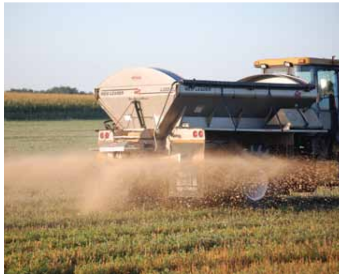
We Energies FGD gypsum can be spread using conventional machinery.
